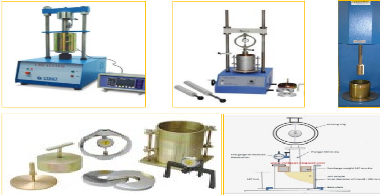
Figure 1: Required equipment for the CBR test
