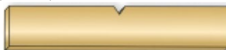
figure 5.4 notched-bar impact specimens form: ISO-V , LxWxH: 55x5x10mm , notch radius: 0,25mm , material: brass
