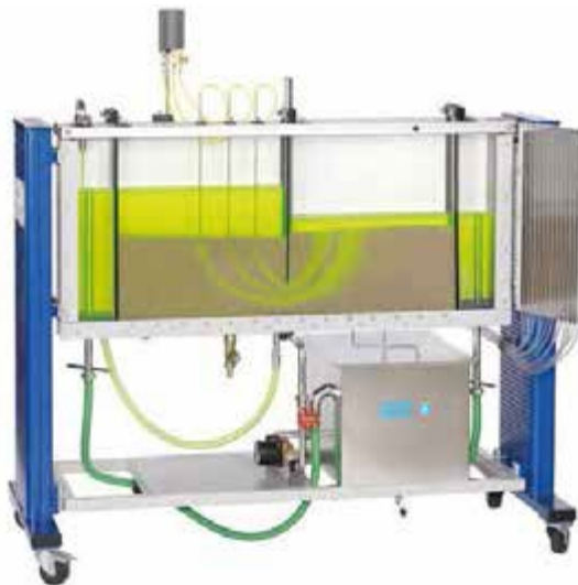
Drainage and Seepage Tank (GUNT-HM 169)
