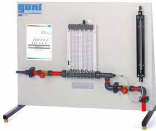
Bernoulli's principle demonstrator (GUNT-HM 150.07)
