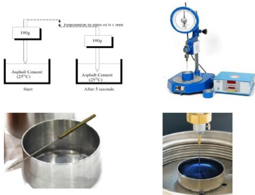
Figure 1: Asphalt penetration apparatus
