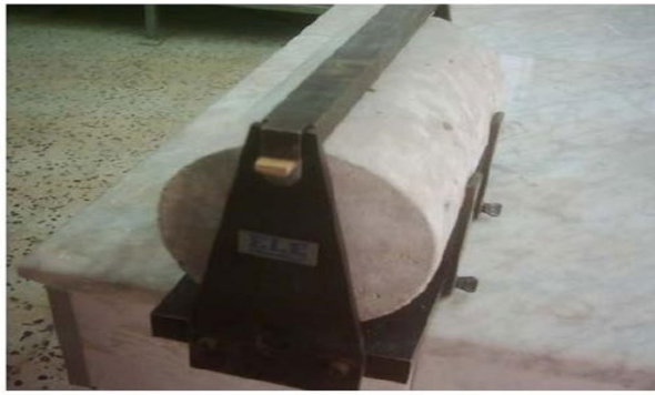
Figure 11: The jig for aligning concrete cylinder and bearing strips
