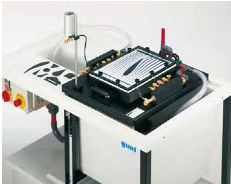
Flow visualization apparatus (GUNT-HM 150.10)
