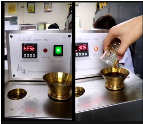
Figure1: Saybolt viscometer and bath
