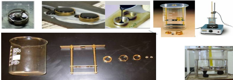
Figure 1: Ring & Ball Apparatus
