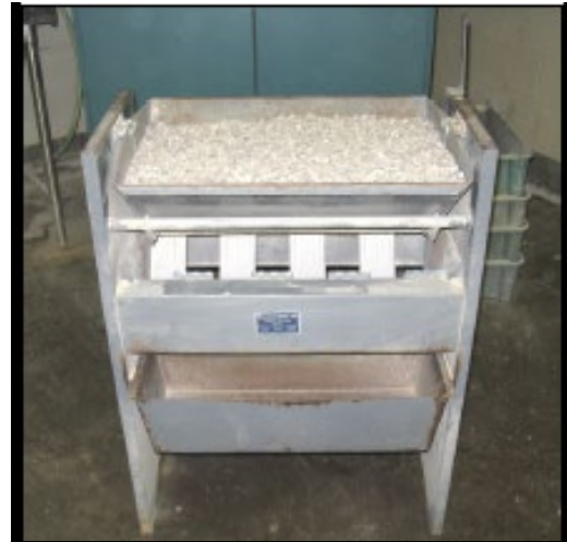
Figure 2: Reducing sample to test size
