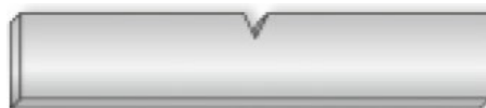
figure 5.3 notched-bar impact specimens form: ISO-V LxWxH: 55x5x10mm notch radius: 0,25mm , material: construction steel
