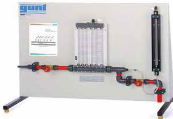
Bernoulli's principle demonstrator (GUNT-HM 150.07)
