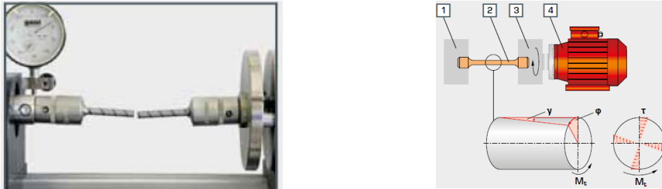
Figure 4.1: Test process in the torsion test ,1 rigid clamping, 2 specimen, 3 rotating clamping, 4 drive; M_t twisting moment, \gamma shearing angle, \phi twisting angle, \tau shear stress
