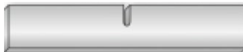
figure 5.5 notched-bar impact specimens form: ISO-U, LxWxH: 55x5x10mm , notch radius: 1mm , material: free cutting steel
