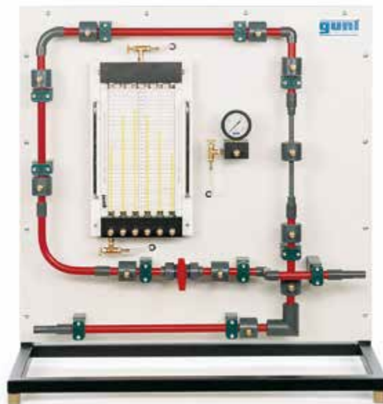
Losses in bends and fittings (GUNT-HM 150.29)
