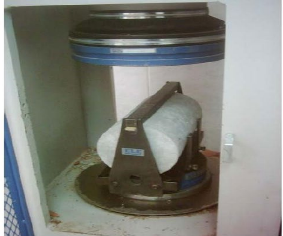
Figure 12: Fitting the cylinder in the compression machine.
